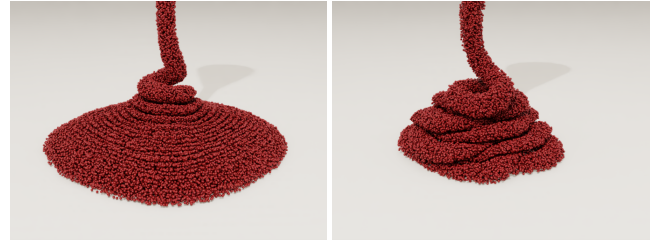
Fig. 18. Viscous fluids with \eta^p = 50\text{Pa}\cdot\text{s} (left) and \eta^p = 500\text{Pa}\cdot\text{s} (right) released from a funnel reservoir form typical coiling patterns.
