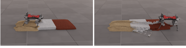
Fig. 13. An ANYmal quadruped walks over a complex terrain with sand, snow and clay according to a pretrained locomotion policy. Two-way coupling between the articulated rigid body solver and MPM terrain forces the robot to change its stride as it progresses through the various materials.
